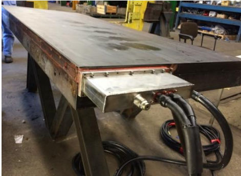
Example instrumented mold plate, with robust optical cable connections
